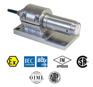
All KIS load cells can be ATEX, IECEx, FM, CSA certified for use in explosive atmospheres.
